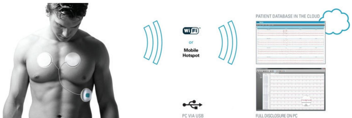
*zensor product wirelessly sends vital signs data using a standard wifi network to a remote database. Full disclosure data can be viewed post-monitoring using viewing software on a PC*
